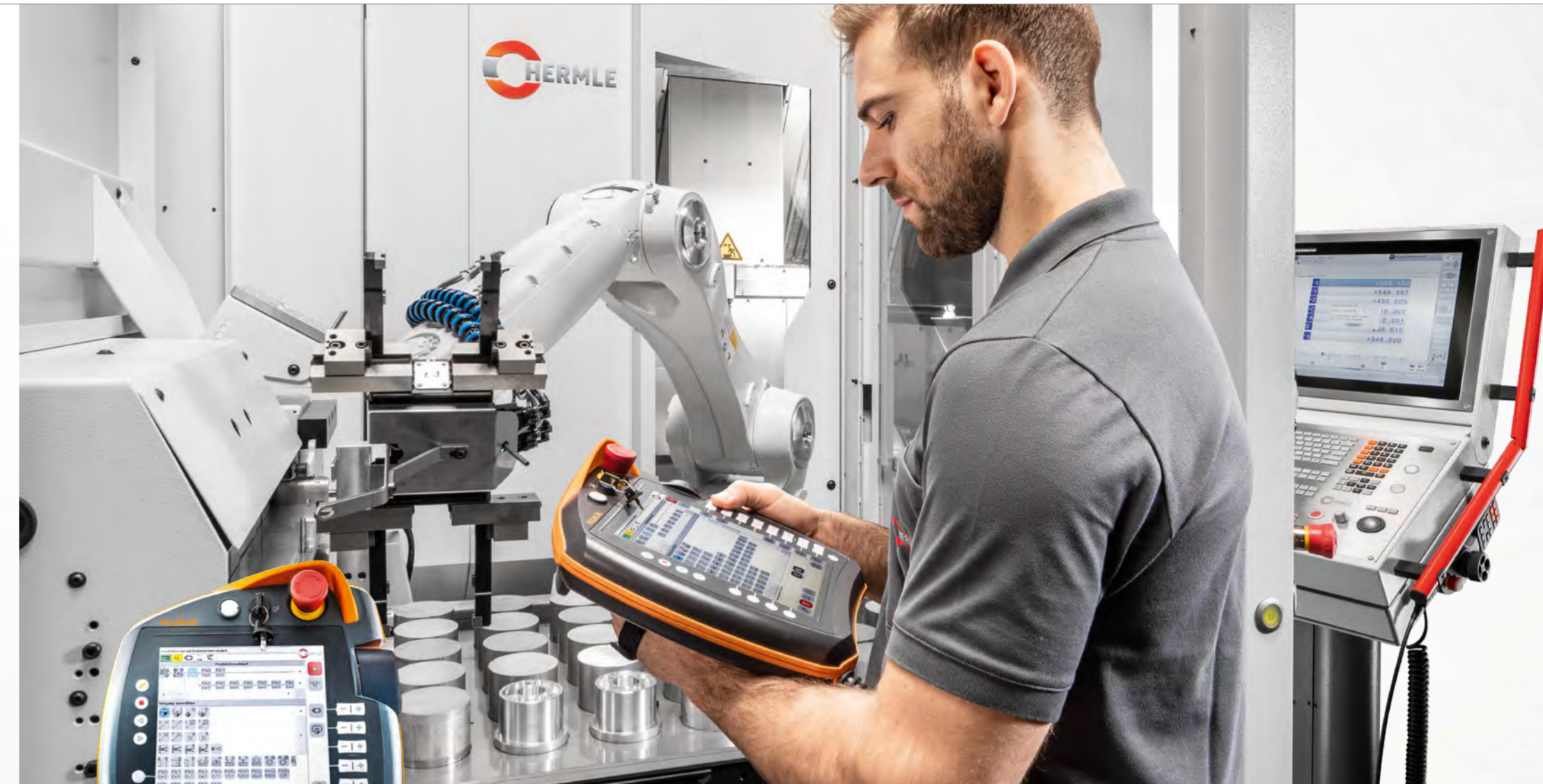
left: Robot operating station SmartPad with touch function for easy robot programming. top: Using graphic robot programming, in short GRP, and simple input values, a wide variety of workpiece blanks are positioned in a space-optimised manner on the dies.
