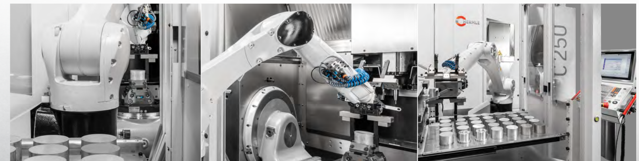
The RS 05-2 robot system adapted to a 5-axis machining centre C 250 of the Performance-Line series.
