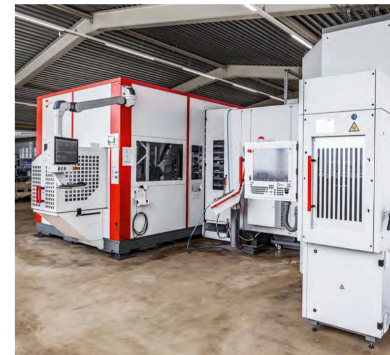
The highly productive flexible C 22 U production cell with the RS 2 robot system (left) and the ZM 192 additional magazine.
