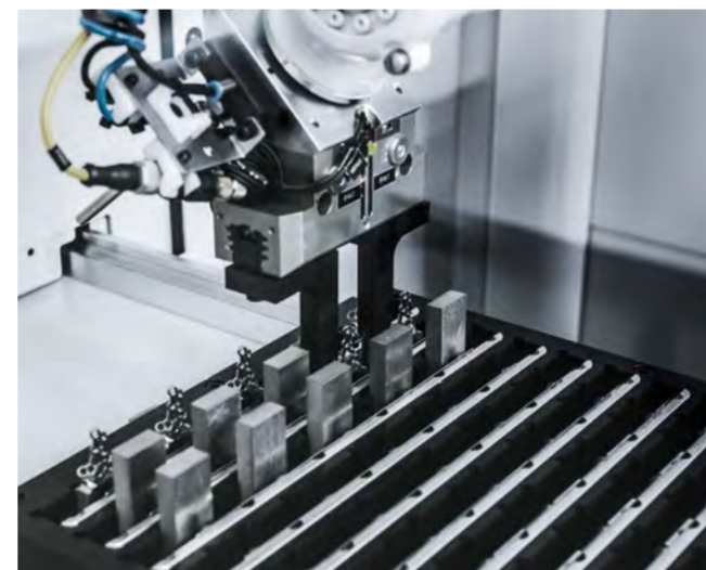
A workpiece pallet designed by Medartis with multiple holding fixtures for supplying titanium blanks or holding finished parts with fully automated robot handling.
