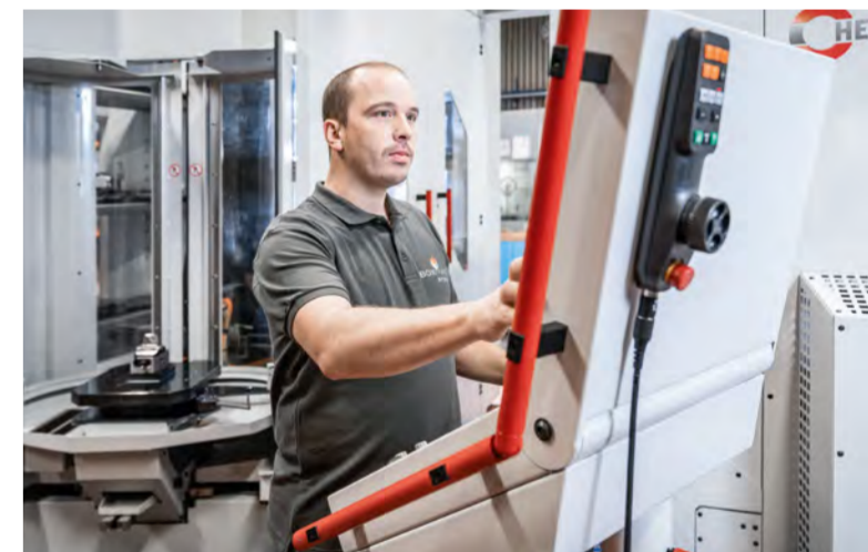
The control comes from Heidenhain (type TNC 640) and is fully digital thanks to the HSCI interface and the EnDat interface.
