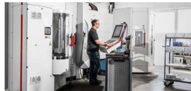
top The Hermle manufacturing cell at HZT Honermeier, consisting of the C 400 U 5-axis machining centre and the HS flex automation solution.
