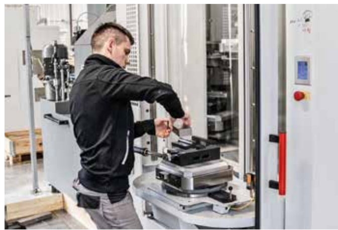
left The C 22 UP has a pallet changing system that allows the operator to set up in parallel to machining time. right Manufacturing complex products means peak precision with materials that are difficult to machine.
