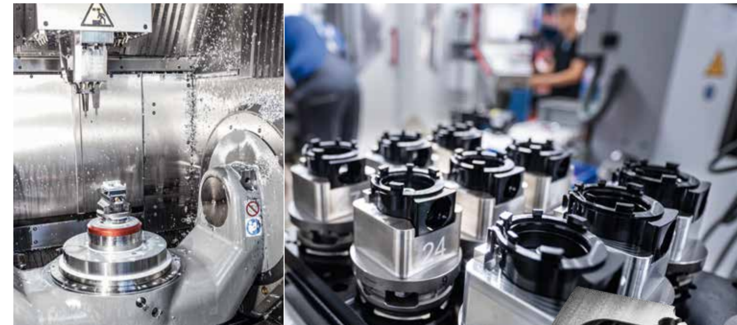
left The C 12 U machines the workpieces for as little as one minute or as much as 1½ hours. right With the new automation capacity, SEPO can also produce precision parts in series. With the HS flex handling system, SEPO has 40 pallets of 240 x 320 millimetres each available for unmanned production. However, 70% of the parts are significantly smaller, like this black anodised aluminium component.
