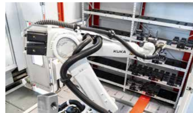
top The RS2 robot stores the dies with the blanks in a storage module until the next C 32 U is ready to process them.
