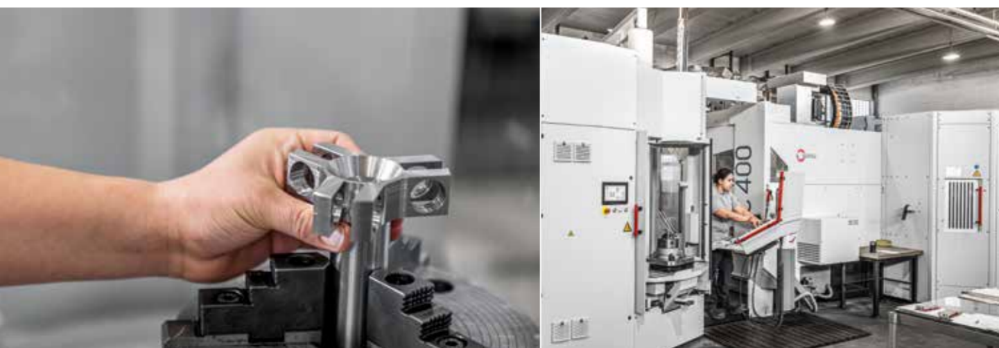
left "Correct clamping of components is very important, otherwise dangerous imbalances develop during the machining process," explains Matthias Reh. right Ergonomic working on the C 400 U: The height of the control panel and tilt of the screen can be optimally adjusted to the operator. The panel is also easy to swing from the magazine loading station to the working area.
