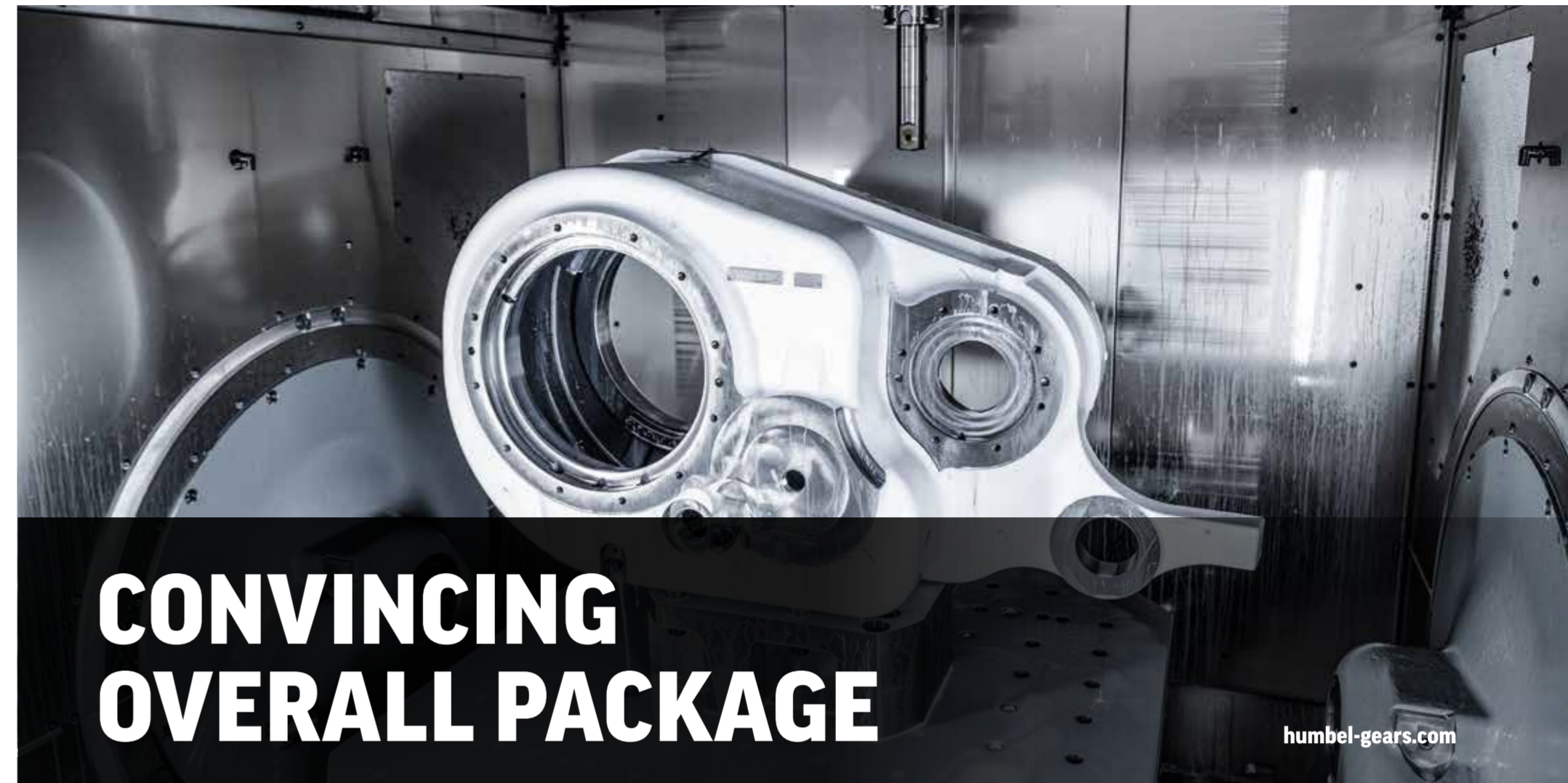
With the C 62 U, Humbel can now also machine the cast housings of railway gearboxes.
