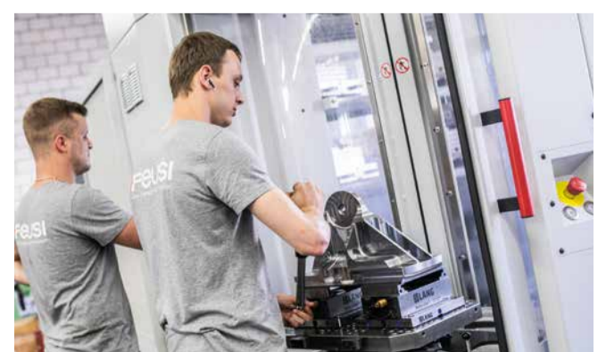
the operator-friendly setup station of the PW 150 pallet changer
