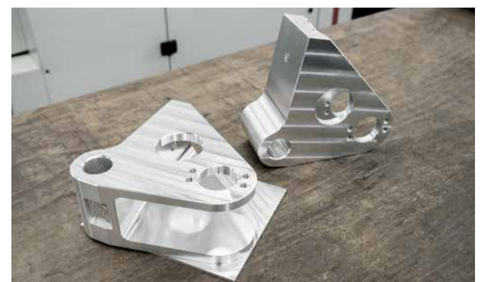
a small excerpt from the range of intricate workpieces made of St 52, CroNiMo 34, stainless steel or aluminium; here, complex chassis parts made of St 52
