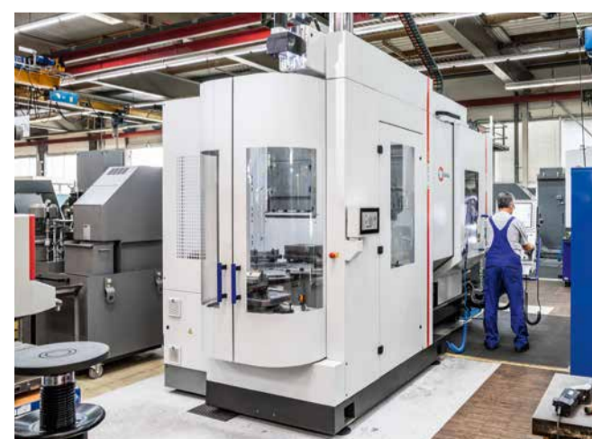
the PW 150 pallet changer of the C 22 UP machining centre; in the foreground is the (rotatable) setup station for loading the pallets/workpiece fixtures with workpieces or for removing the finished parts
