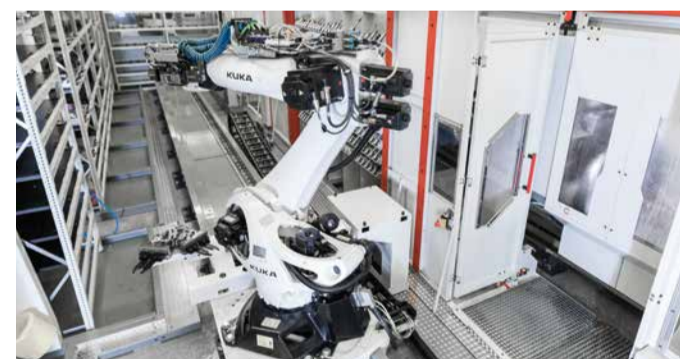
the perspective top view of the flexible manufacturing cell with the magazine area for workpiece pallets (left and rear), the magazine for the 200 tools on the right in the sub-area, the connection of a machining centre C 42 U on the right at the front and the robot in the middle, which, as a multifunctional system, is responsible for handling both the workpiece pallets and changing the tools
