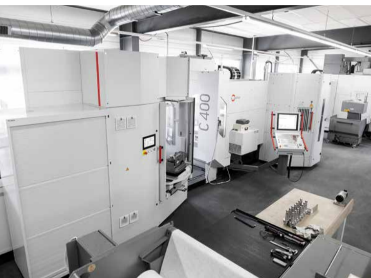
The image shows a part of the "Hermle Boulevard" at Feusi AG, featuring the 5-axis machining centre C 400 U with workpiece magazine, the 5-axis machining centre C 22 U with pallet changer PW 150 and the 5-axis machining centre C 42 U/MT with rotary functionality
