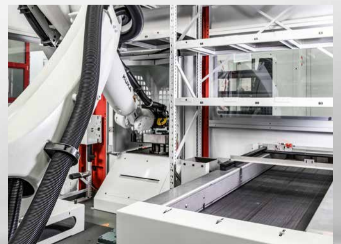
Pallet storage, setup station (rear) and conveyor belt for workpieces
