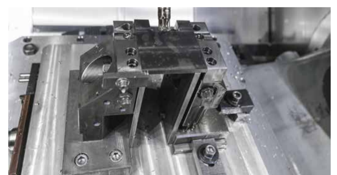
the working area of a 5-axis CNC high-performance machining centre C 42 U with swivelling rotary table measuring 800 x 630 mm in diameter and a clamping device clamped on a pallet for the 5-axis machining of a workpiece
