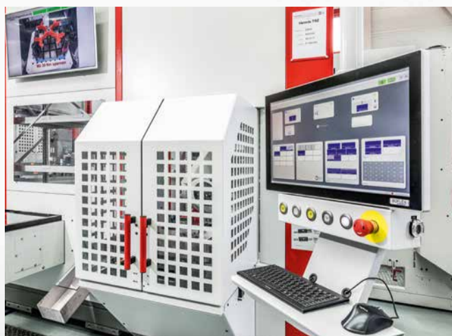
RS 2 Combi robot system with kanban, adapted to a C 32 U dynamic 5-axis machining centre
