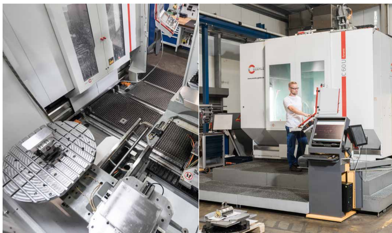
left The pallet change system of the highly flexible 5-axis CNC high-performance machining centre C 42 UP for "round-the-clock" complete production of mould plates, mould superstructures and active parts for the mechanical engineering and tool construction industry right The 5-axis CNC high-performance machining centre C 60 U for large parts.
