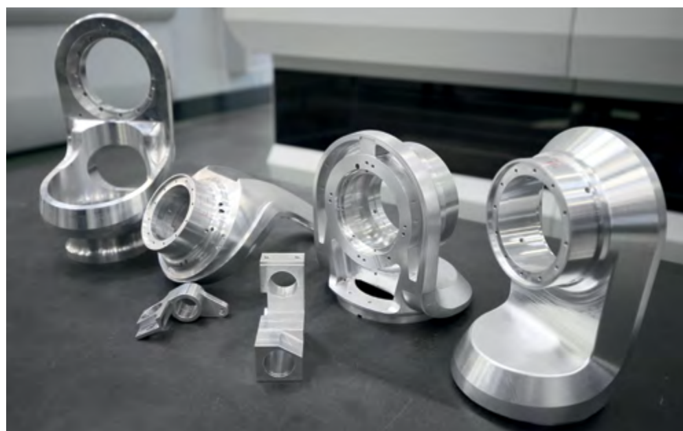
Robot components in various sizes that are fully manufactured on the twelve new Hermle C 42 UP machining centres
