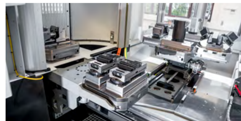
The PW 250 pallet changer with storage (rear right) and the setup station (left); including the pallets in the working area, there are seven pallets in the system that can be loaded with the same or different multiple clamping fixtures and/or workpieces
