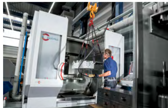
Shows the simple crane loading procedure for a C 60 U machining centre with the double doors open
