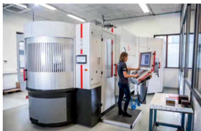
Overall view of the high-performance, 5-axis Hermle C 32 U CNC machining centre with a PW 250 pallet changer with storage; the PW 250 setup station is located at the front
