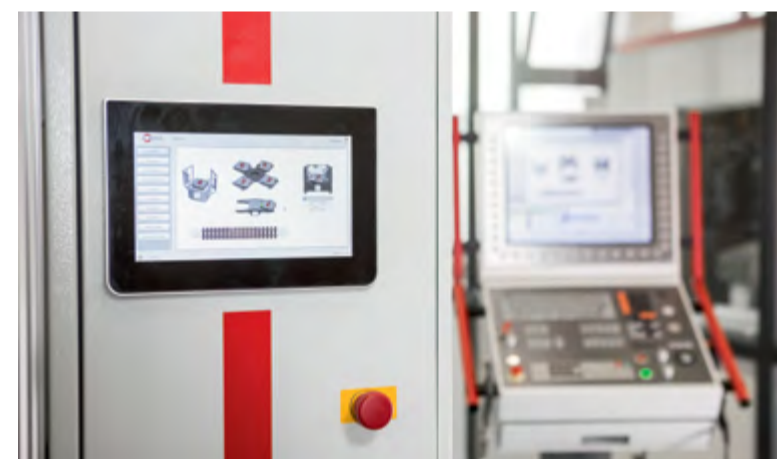
The additional display at the setup station of the PW 250 pallet changer for quick registration and visual monitoring of the process sequences and pallet information stored in the HACS
